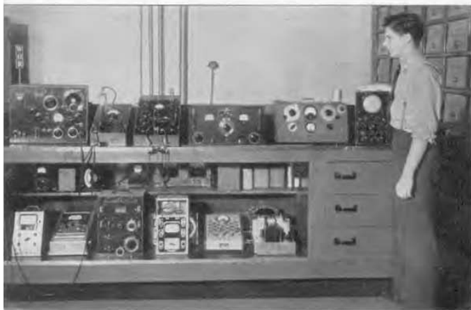
FIGURE 3. Equipment used on the test bench includes impedance bridges, vacuum-tube voltmeters, standard-signal generators, and other general-purpose test instruments.
