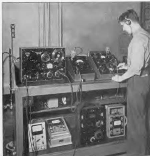
FIGURE 4. Another view of the test bench showing the TYPE 650-A Impedance Bridge in use.
